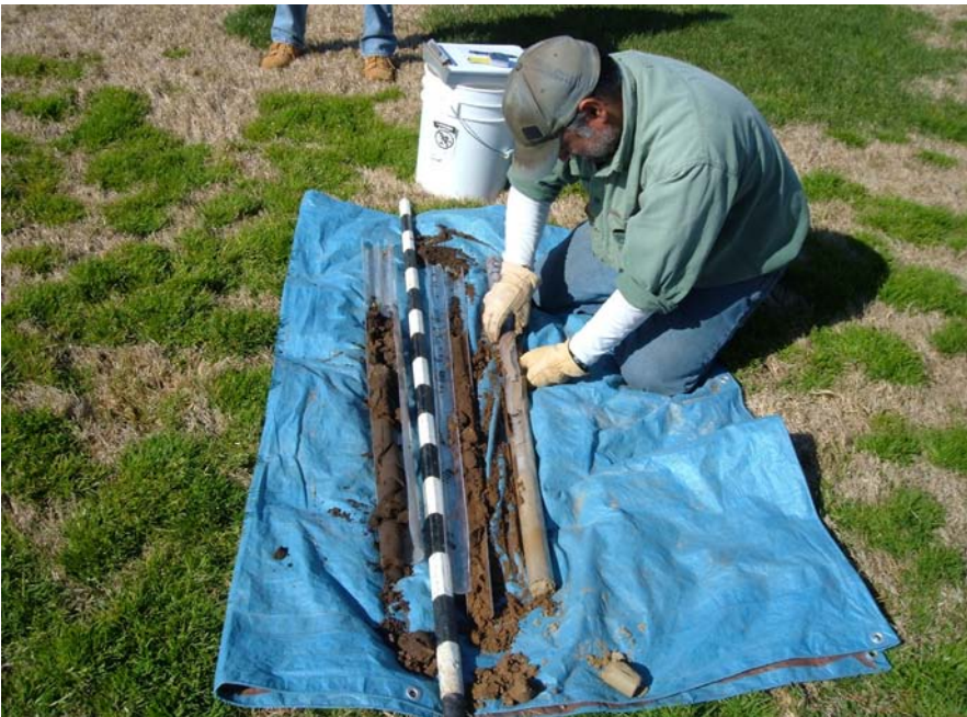
Geoprobos used to conduct the archaeology study prior to the treatment plant upgrade project.
