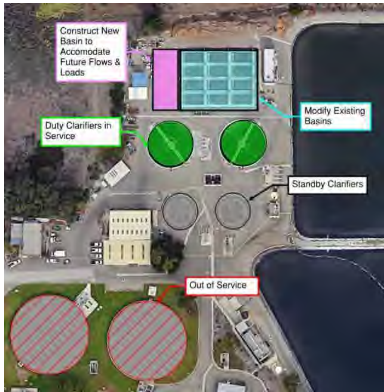
Figure 4-2: Conceptual Site Layout for MLE
