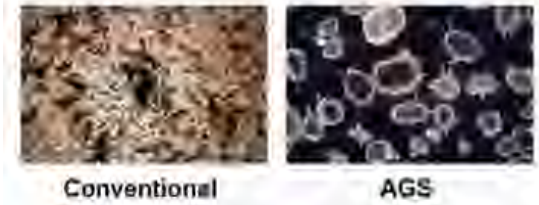
Conventional floc vs AGS granules
