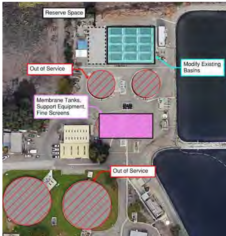
Figure 4-11: Conceptual Site Layout for MBR
