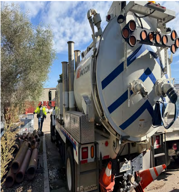
Photo 25: Inspection (combination truck)
