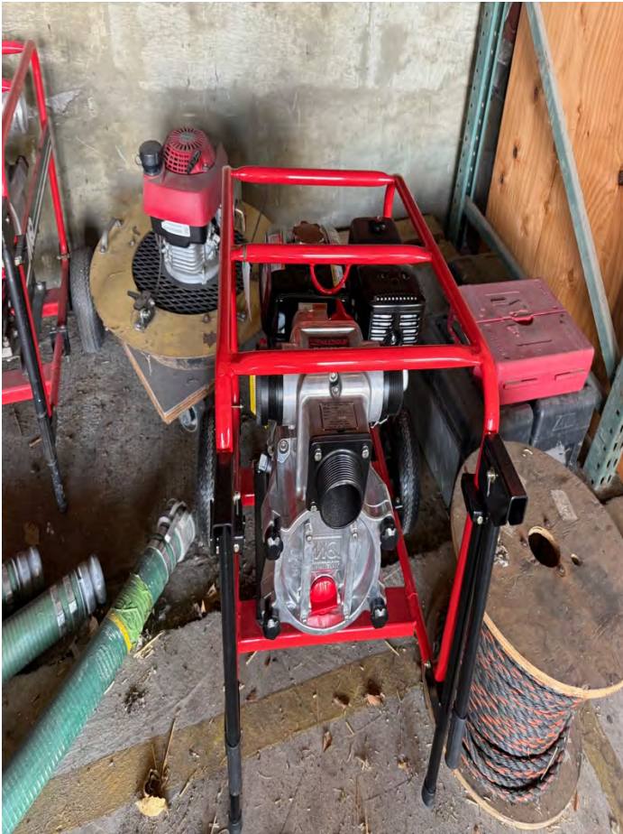
Photo 29: Inspection (trash pump)
