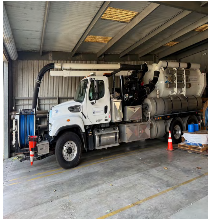
Photo 26: Inspection (combination truck)
