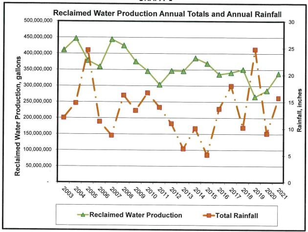
Higher volumes of reclaimed water are produced during the dry summer months when the reclaimed water demand for irrigation is greatest due to the lack of rainfall and hotter weather patterns. During 2021, the maximum reclaimed water production occurred in July, when over 47 million gallons were produced. The lowest months for reclaimed water production occurred during November and December. An increase in production occurred during April through September to meet the demand.
