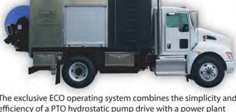
The exclusive ECO operating system combines the simplicity and efficiency of a PTO hydrostatic pump drive with a power plant that operates at lower RPM than traditional designs. Trucks equipped with ECO options experience less engine wear and lower fuel consumption, saving operators time and money.
