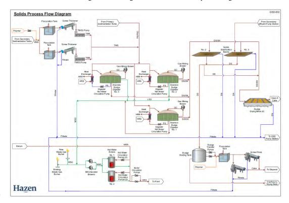
Figure 1. Solids Process Flow Diagram
